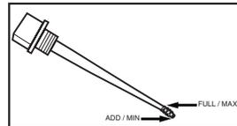
Be sure the machine is level when checking the oil level. (Refer to the engine operating manual for seasonal grades).
